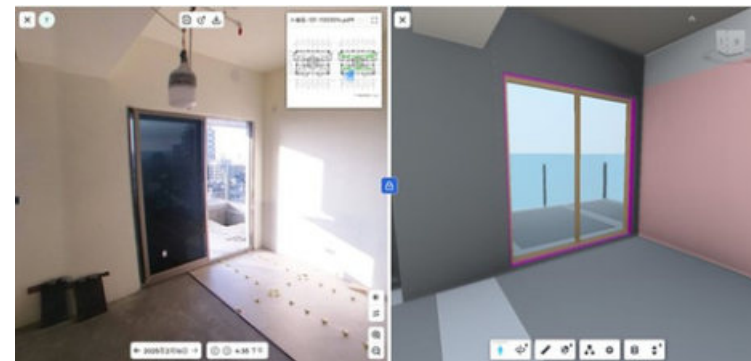
The BIM model can be compared to the actual construction process and results to verify that the construction is being performed in accordance with the verified design conclusions.
